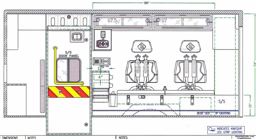
DOOR INTERIOR DIMENSIONS NOTES HEIGHT WIDTH DEPTH NO. 8.50" SLIDING POLY DOORS, RESTOCKING 11.00 44.00 U7.5 11.00 44.00 8.50 SLIDING POLY DOORS, RESTOCKING
