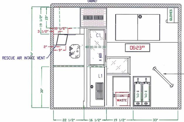
BULKHEAD WALL BUILT OUT FOR RECESSED STORAGE OF D-CYLINDERS AND TRASH
