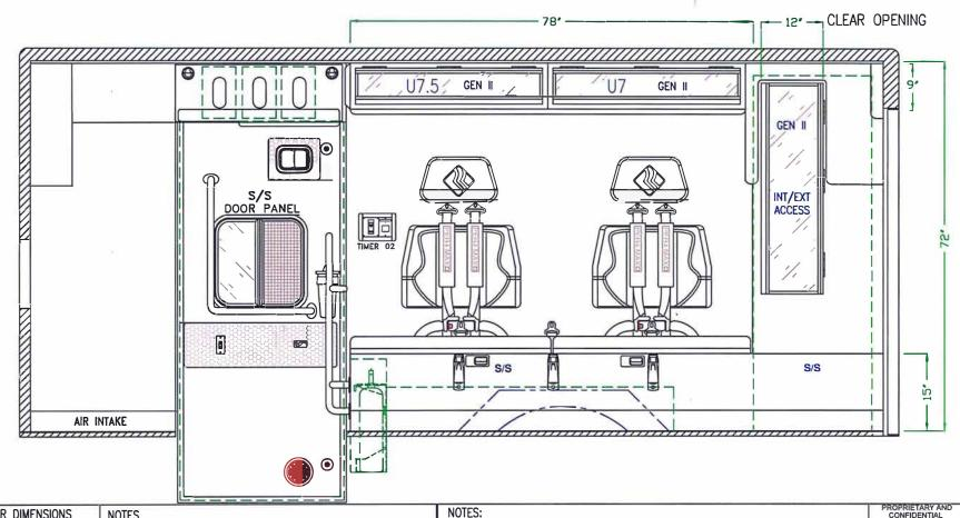
DOOR INTERIOR DIMENSIONS NOTES HEIGHT WIDTH DEPTH FLIP UP GEN II DOOR, RESTOCKING 8.50" 9.00" 40.00 U7.5 9.00" 38.00 8.50" FLIP UP GEN II DOOR, RESTOCKING
